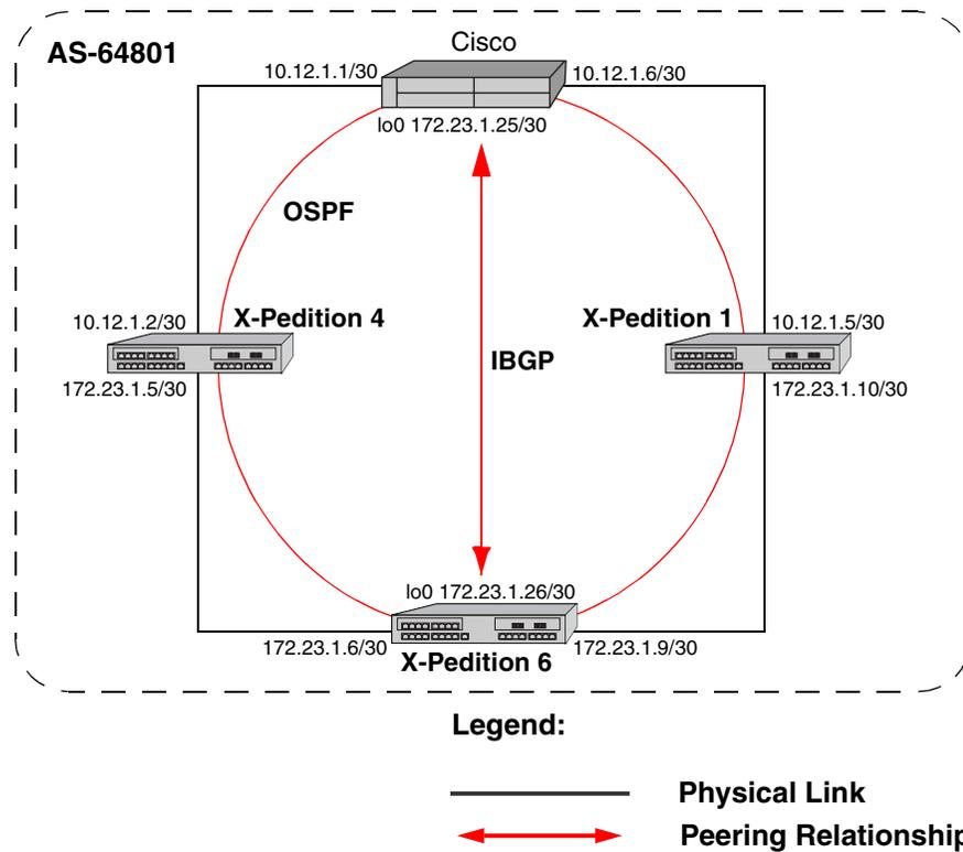
Figure 24. Sample IBGP Configuration (Routing Group Type)
