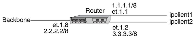
Traffic from two interfaces, ipclient1 with IP address 1.2.2.2 and ipclient2 with IP address 3.1.1.1, is restricted to 10 Mbps for each flow with the following configuration:
