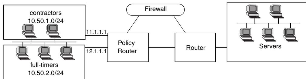
**Figure 38. Using an IP Policy to Authenticate Users Through a Firewall**
