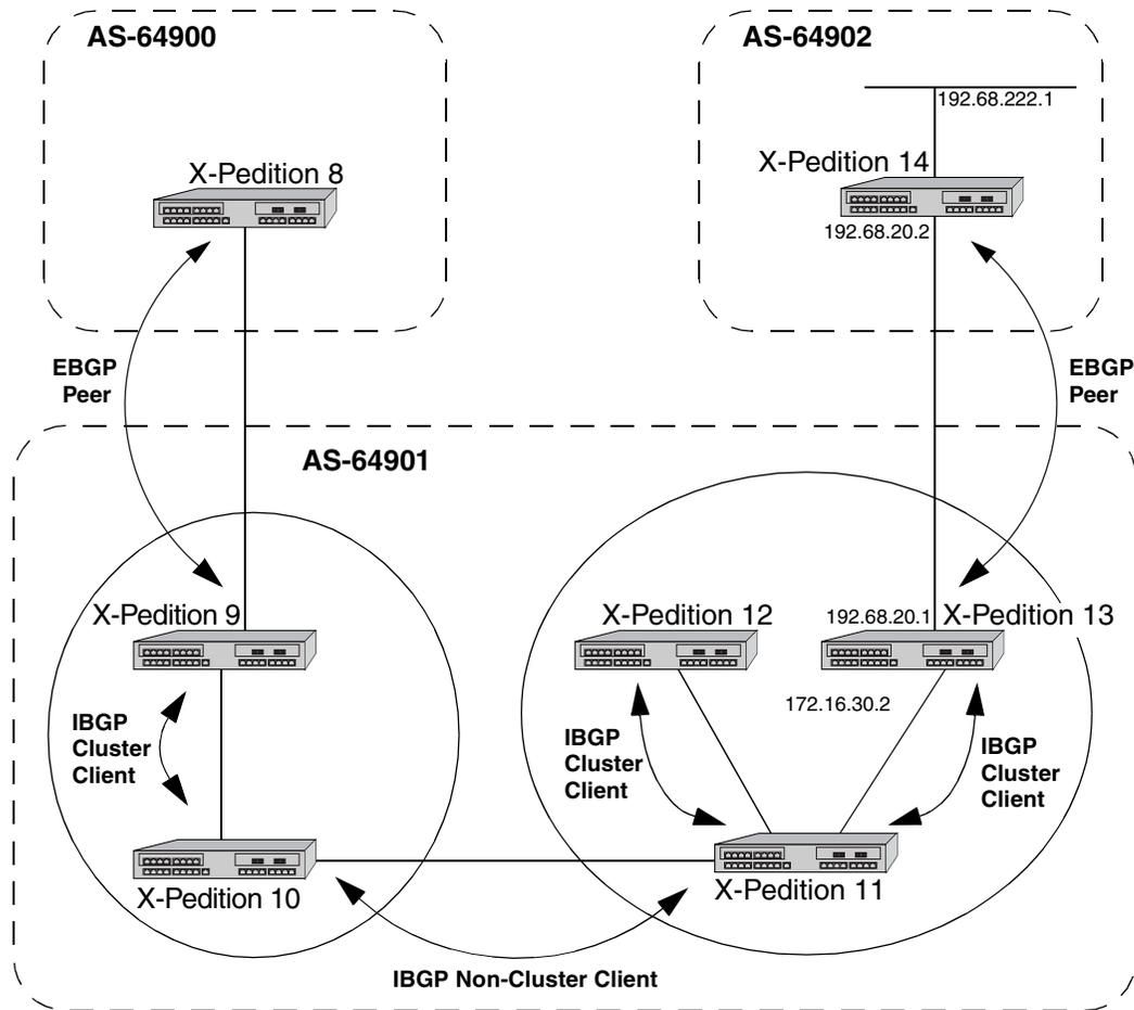
Figure 31. Sample BGP Configuration (Route Reflection)
