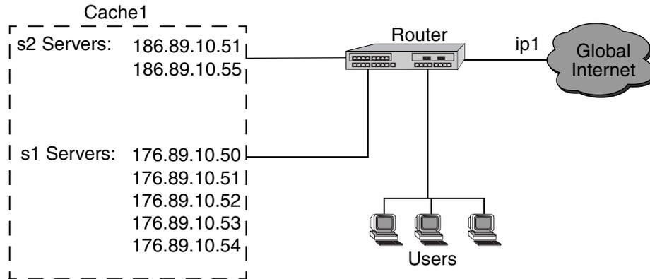
The following commands configure the cache group 'cache1' that contains the servers shown in the figure above and applies the caching policy to the interface 'ip1':
