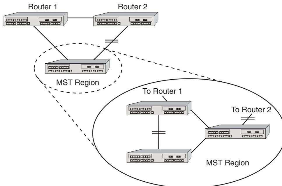
For a device to be considered as part of an MST region, it must be administratively configured with the same Configuration Identifier information as all other devices in the MST Region. The Configuration Identifier consists of four separate parts:
