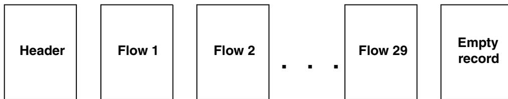
As demonstrated in the following figure, when flows 30 and 31 terminate, each termination results in the creation of an export record. Since the record for flow 30 fills the export buffer, data for flows 1-30 exports to a collector.
