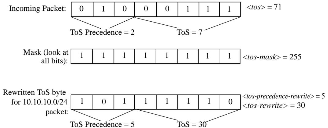
The `<tos-mask>` value determines the ToS bit to be examined, which is all eight bits in this example. The following command configures the ToS rewrite for the example:
