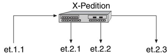
Port et.1.1 is being mirrored out 3 ports, et.2.1, et.2.2 and et.2.3.
