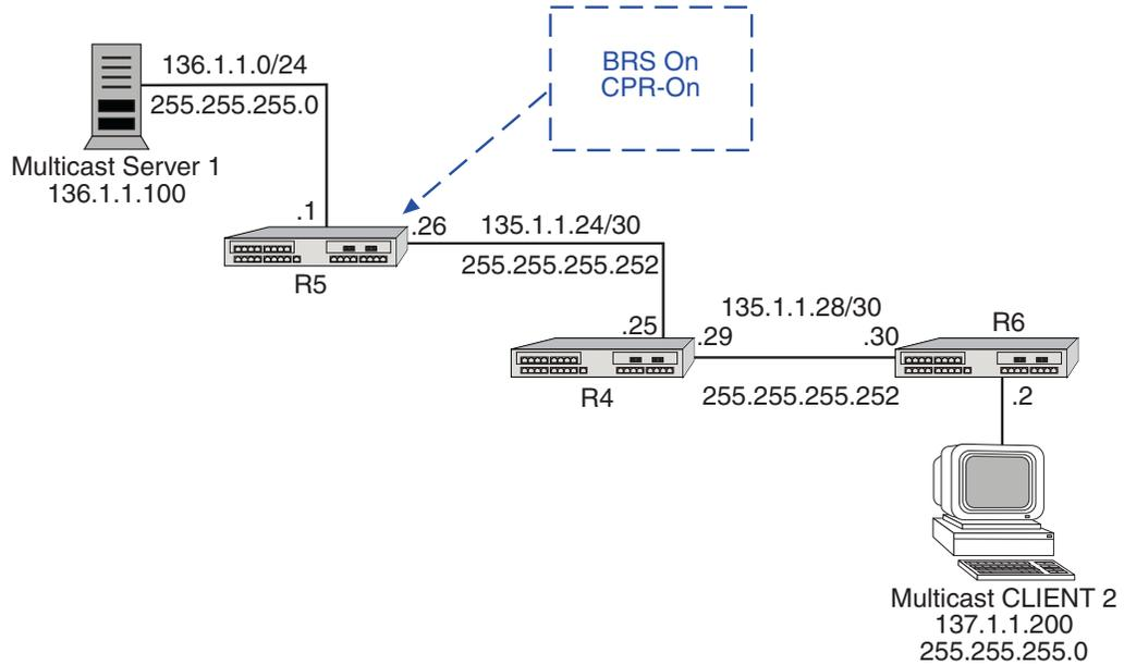
**Figure 34. Using RIPv2, OSPF, and BGP to provide route information for PIM-SM**
