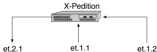
The following command will redirect unlearned traffic for ports et.1.1 and et.1.2 to port et.2.1 after the unlearned traffic rate reaches 2 Kpkts/sec for 30 sec. The traffic will be redirected for the default time of 5 min.
