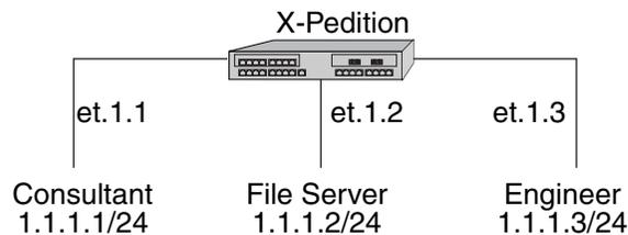
**Figure 41. Sample VLAN for Layer-4 bridging**
