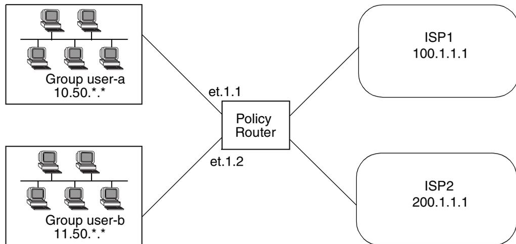
**Figure 36. Using an IP Policy to Route Traffic to Two Different ISPs**
