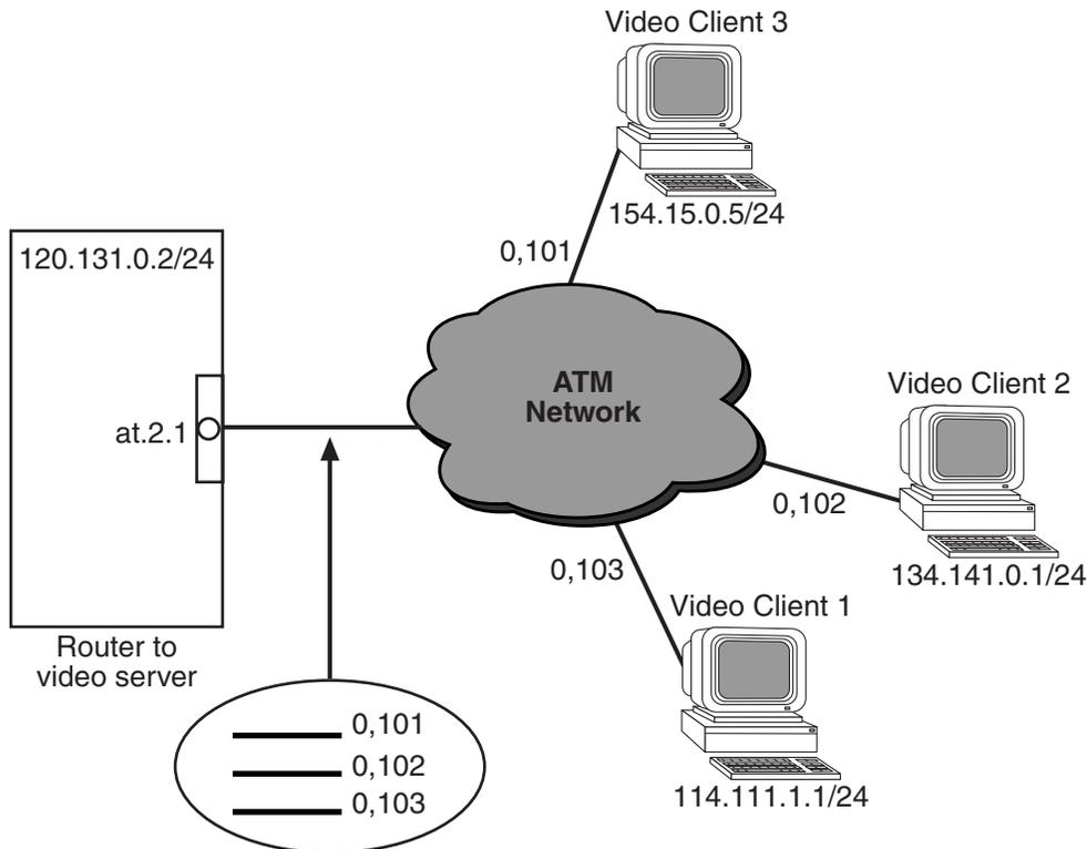
Suppose you wish to set up a connection between a video server and 3 video clients. The video server will route data through the router to the 3 separate video clients (Video Client 1, Video Client 2, and Video Client 3). The requirement is to pass traffic to the video clients through 3 separate virtual channels. This will allow you to apply a unique service profile to each Client's connection.
