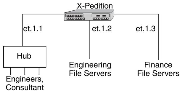
**Figure 40. Source Filter Example**
