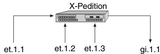
Ports et.1.1, et.1.2 and et.1.3 are being mirrored out gi.1.1
