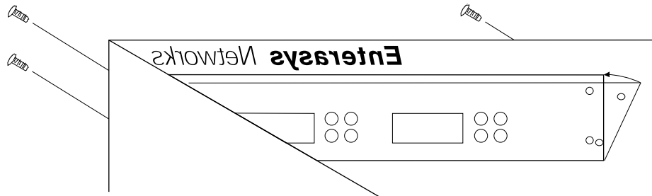
Figure 12. Installing the new face plate (view from inside chassis)
