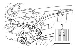
1. Brake pad wear indicator groove
