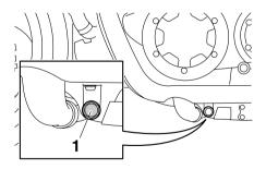
1. Engine oil drain bolt
