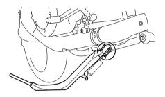
The operation of the sidestand should be checked before each ride, and the sidestand pivot and metal-to-metal contact surfaces should be lubricated if necessary.
