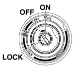
The main switch/steering lock controls the ignition and lighting systems, and is used to lock the steering. The various positions are described below.
