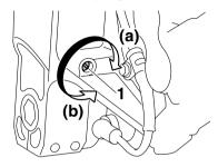
Compression damping force adjusting screw
