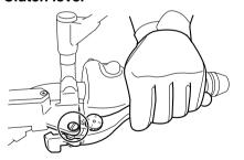
The operation of the brake and clutch levers should be checked before each ride, and the lever pivots should be lu-
