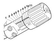
To increase the spring preload and thereby harden the suspension, turn the adjusting knob in direction (a). To decrease the spring preload and thereby soften the suspension, turn the adjusting knob in direction (b).
