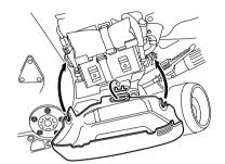
2. Turn the key counterclockwise to the original position, and then remove it.
