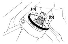
1. Spring preload adjusting bolt
