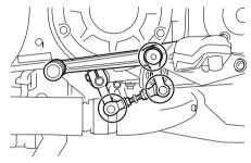
The operation of the shift pedal should be checked before each ride, and the shift pedal rod pivots should be lubricated if necessary.
