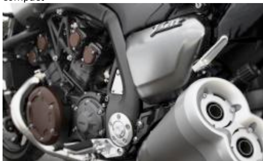
Magnesium engine covers and titanium mufflers
