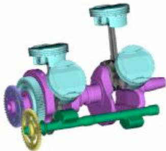
After extensive testing: the V-cylinder angle is more narrow
